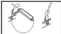
2) For Fixed mode, rotate black block parallel to crampon. Slide notch at back of crampon under heel pad. Holes of crampon line up with touring bracket holes. Slide pin through and secure binding and crampon.
